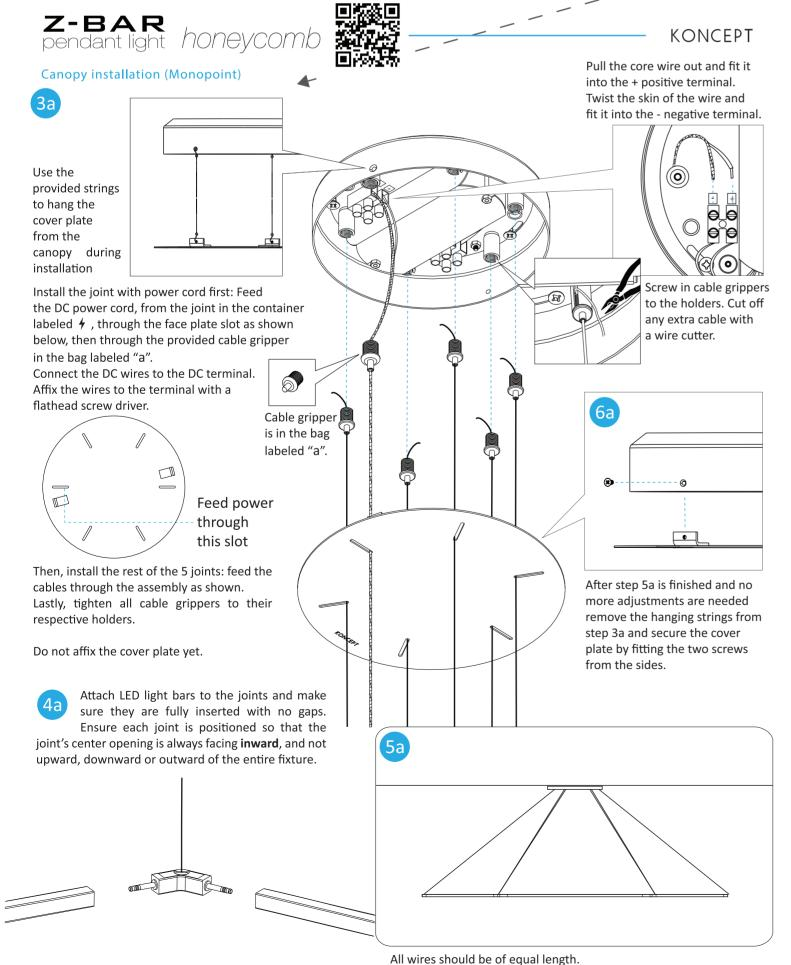
Wires can be released and re-adjusted by pressing in the cable
