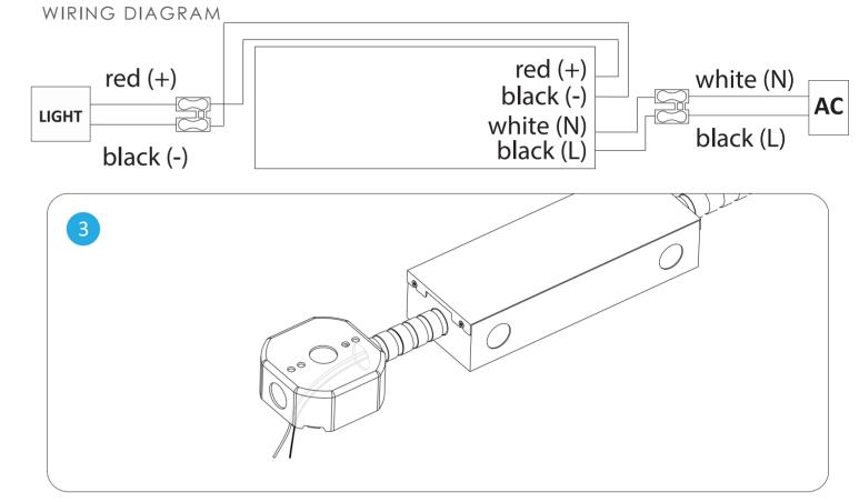
Feed the Red and Black DC wires through the conduit into the junction box (conduit and junction box not provided). Affix the transformer enclosure and junction box properly inside the ceiling, with an opening allowing access to the junction box.
