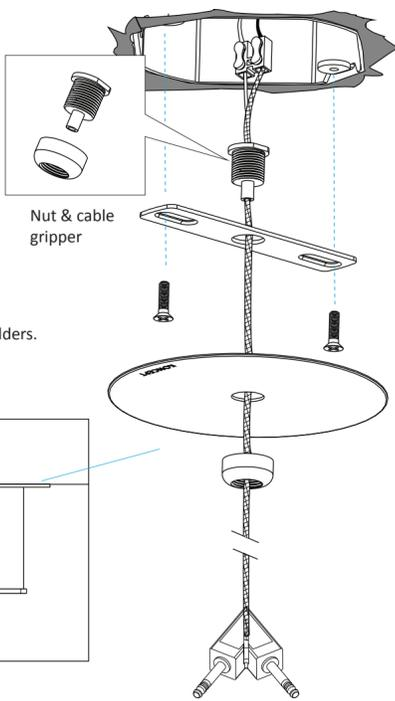
Affix the rectangular metal holder with the two provided screws to the junction box, then install the cover plate by tightening the nut to the cable gripper.
