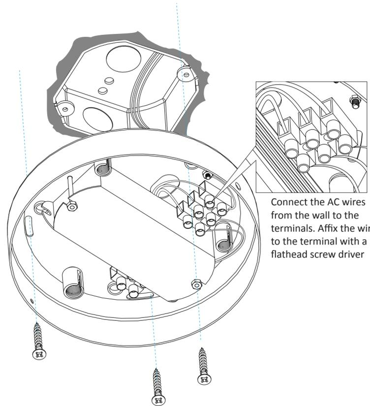
Connect the AC wires from the wall to the terminals. Affix the wires to the terminal with a flathead screw driver
