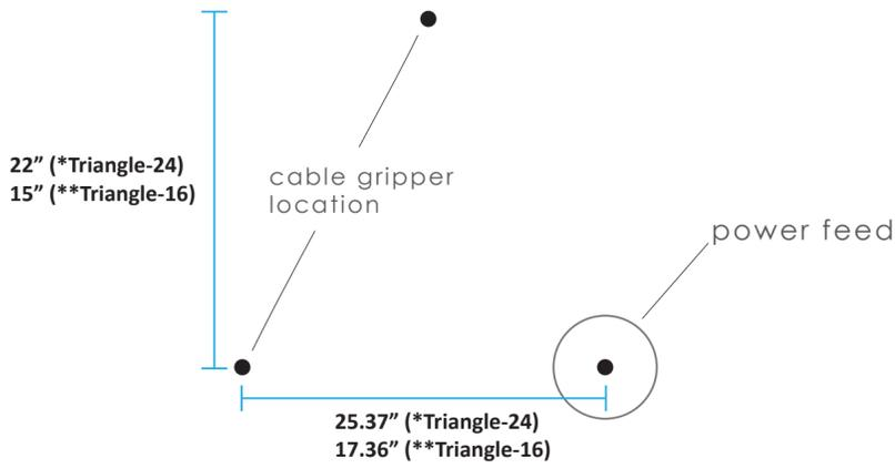
\* measurements for Triangle-24 fixture
