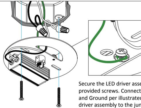
Secure the LED driver assembly using the provided screws. Connect Hot, Neutral and Ground per illustrated and affix LED driver assembly to the junction box
