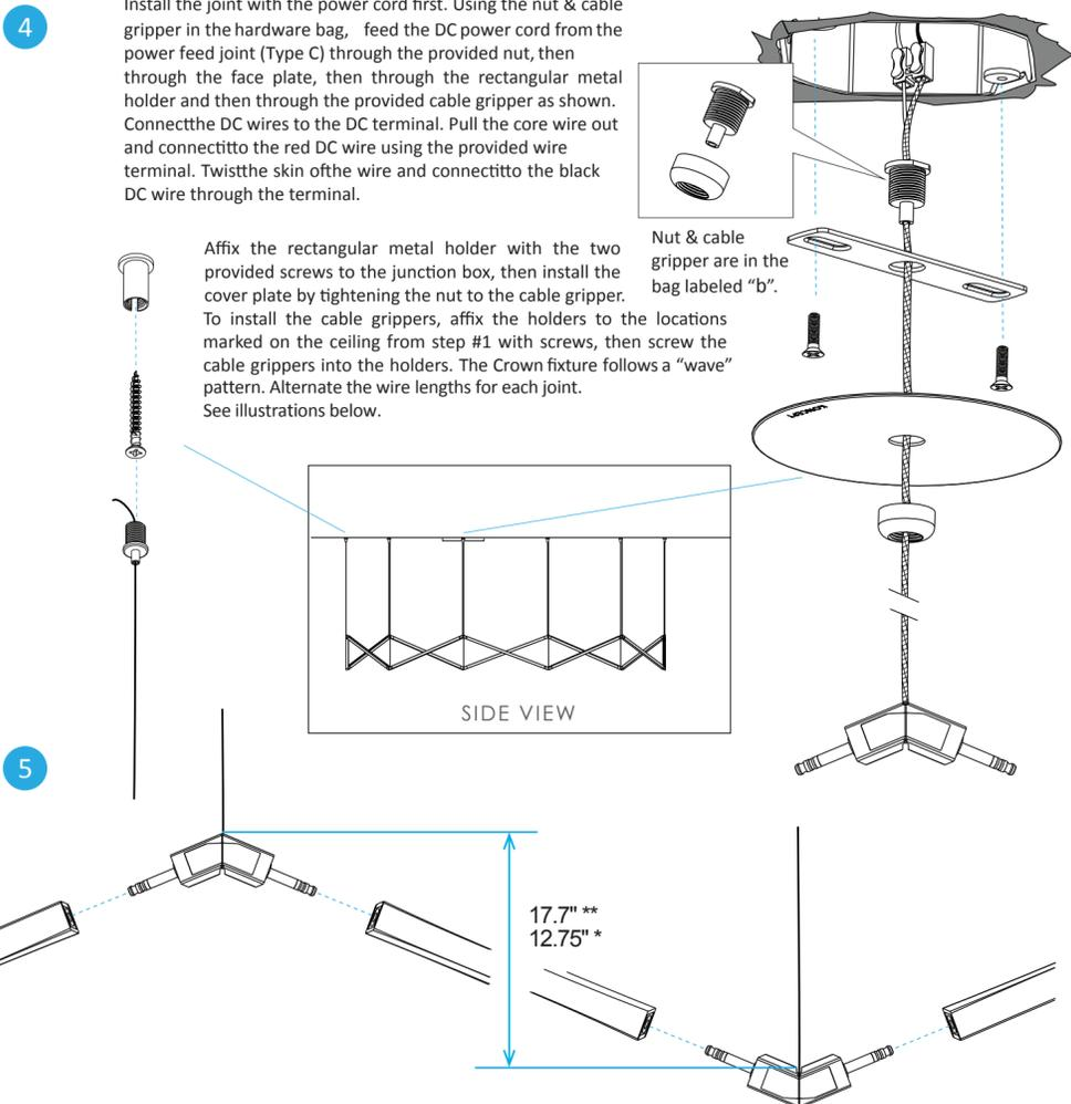
\* measurements for Crown-36 fixture
