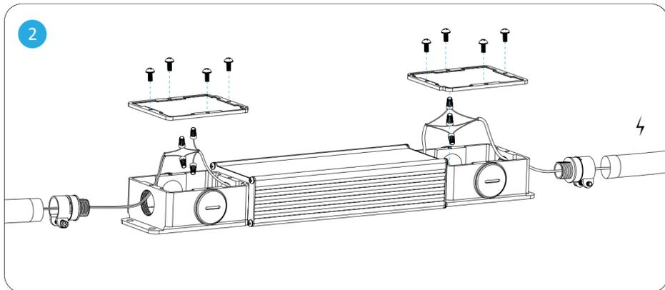
Using the provided DC cable & connectors, connect the wires inside the transformer enclosure as illustrated in the Wiring Diagram below.
