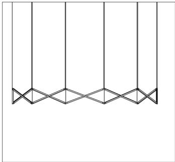
Before installing the pendant light, map out the installation points on the ceiling according to the measurements shown below. The Z-Bar pendant light will be hung vertically from each of the joints.
