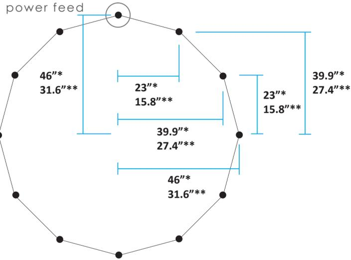
\* measurements for Crown-24 fixture
