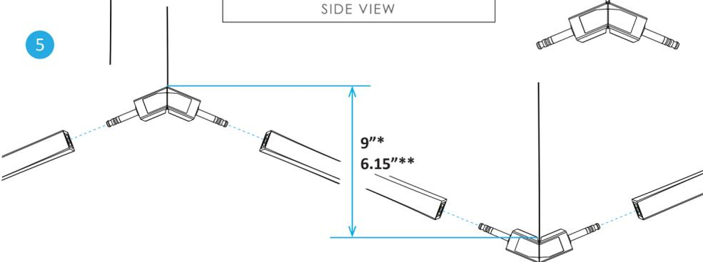
Attach the LED light bars to the joints making sure they are fully inserted with no gaps between the light bars and the joints. Ensure every joint is positioned so that its center opening is always facing inward, and not upward, downward or outward of the entire fixture.
