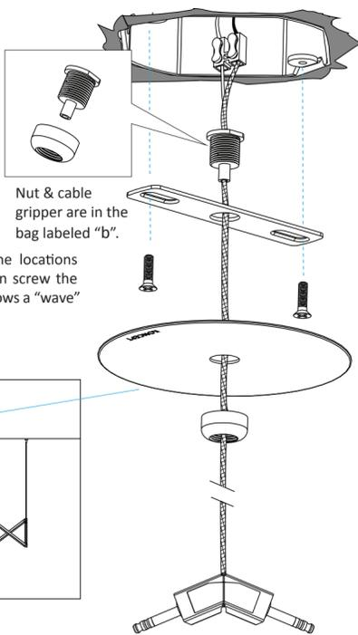
Affix the rectangular metal holder with the two provided screws to the junction box, then install the cover plate by tightening the nut to the cable gripper. To install the cable grippers, affix the holders to the locations marked on the ceiling from step #1 with screws, then screw the cable grippers into the holders. The Crown fixture follows a "wave" pattern. Alternate the wire lengths for each joint. See illustrations below.
