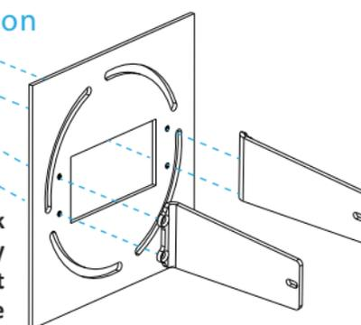
2 Using the provided screws, install the mounting arms as illustrated.
