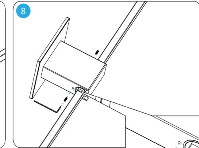
Using the provided hex key, screw in the two lock screws on both sides. Rotate the LED light bar to direct the light as you wish.
