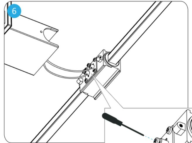
Connect the +positive (RED) and the -negative (BLACK) wires from the LED driver to the +positive and -negative wiring terminals on the lamp accordingly.
