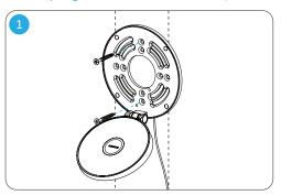
Installation of the Gravy Wall Sconce on a wood stud is recommended. Locate a wood stud using a wood stud finder device. Using the provided screws, secure the Gravy Wall Sconce to the wood stud.
