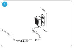
Connect power supply to the lamp cable, then plug in the power supply to a wall outlet.
