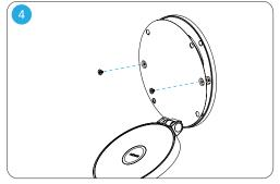
Secure the round metal plate to the Gravy Wall Sconce with screws.
