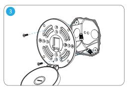
Secure Gravy Wall Sconce to the junction box with screws. A junction box of at 1.5" depth should be used so that the LED driver will fit. LED driver should be completely seated inside the junction box.
