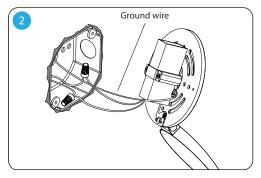
Using the provided cable connectors, connect the wires as illustrated in the Wiring Diagram on the next page.
