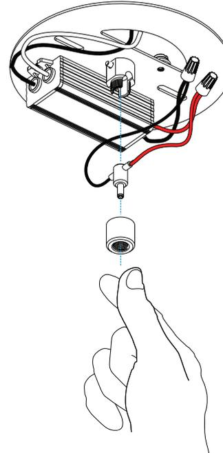
Connect the T-shape connector to the LED driver by connecting the red and black wires to the LED driver respectively. Place it in the receiving holder in the canopy, and screw in Strain relief knob to hold it in place.
