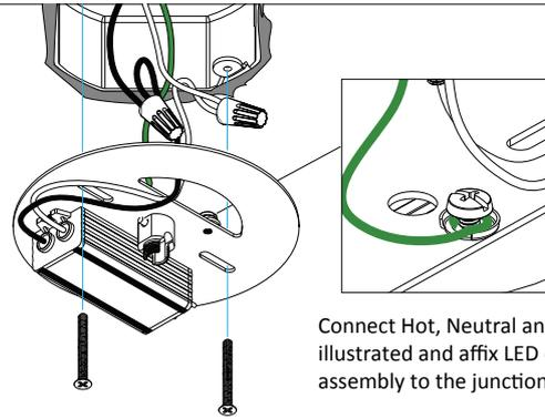
Connect Hot, Neutral and Ground per illustrated and affix LED driver assembly to the junction box
