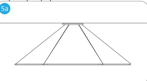
Adjust wires (press cable gripper's nozzle) so that all are of equal length. Please make sure the minimum cable lengths are: 32 inches for the 24" model, and 22 inches for the 16" model.
