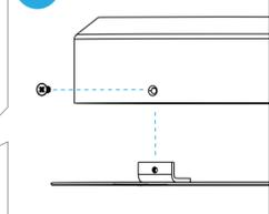
After step 5a is finished and no more adjustments are needed remove the hanging strings from step 3a and secure the cover plate by fitting the two screws from the sides.
