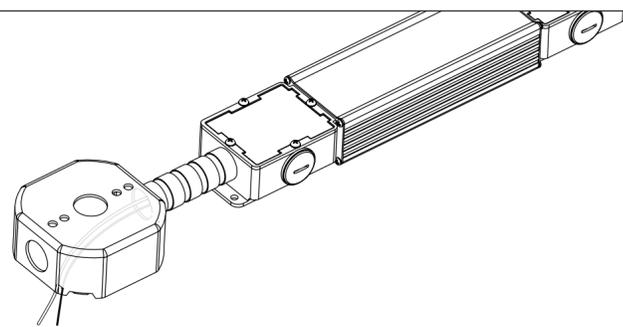
Feed the Red and Black DC wires through the conduit into the junction box (conduit and junction box not provided). Affix the transformer enclosure and junction box properly inside the ceiling, with an opening allowing access to the junction box.
