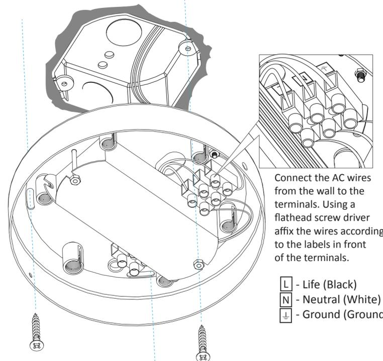
Feed the AC power cord from the junction box through the hole as shown in the figure on the right then connect the AC wires to the terminals. Use a flathead screw driver to tighten the screws in the terminal to affix the wires. Secure the canopy to the ceiling with 3 provided screws, make sure the canopy is centered to the junction box and fully covering the junction box.
