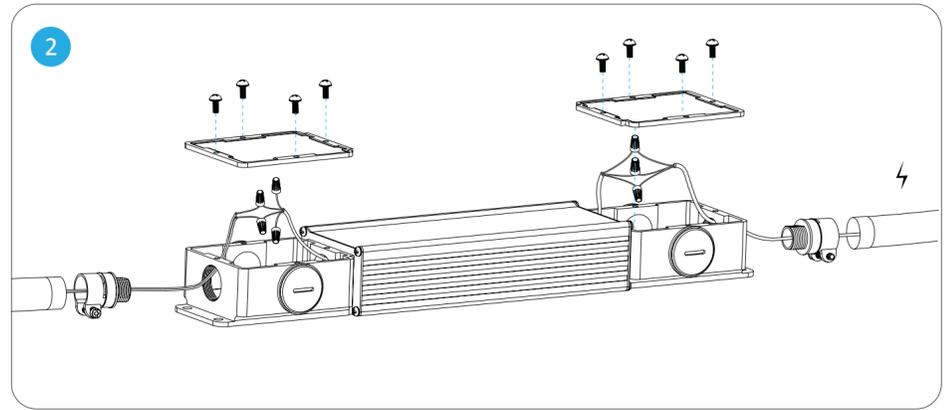
Using the provided DC cable & connectors, connect the wires inside the transformer enclosure as illustrated in the Wiring Diagram below. A transformer needs to be installed for every location marked with the symbol (J)
