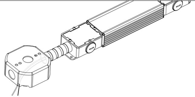
Feed the Red and Black DC wires through the conduit into the junction box (conduit and junction box not provided). Affix the transformer enclosure and junction box properly inside the ceiling, with an opening allowing access to the junction box.
