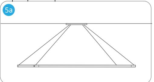
Adjust wires (press cable gripper's nozzle) so that all are of equal length. Please make sure the minimum cable lengths are: 23 inches for the 24" model, and 15 inches for the 16" model.
