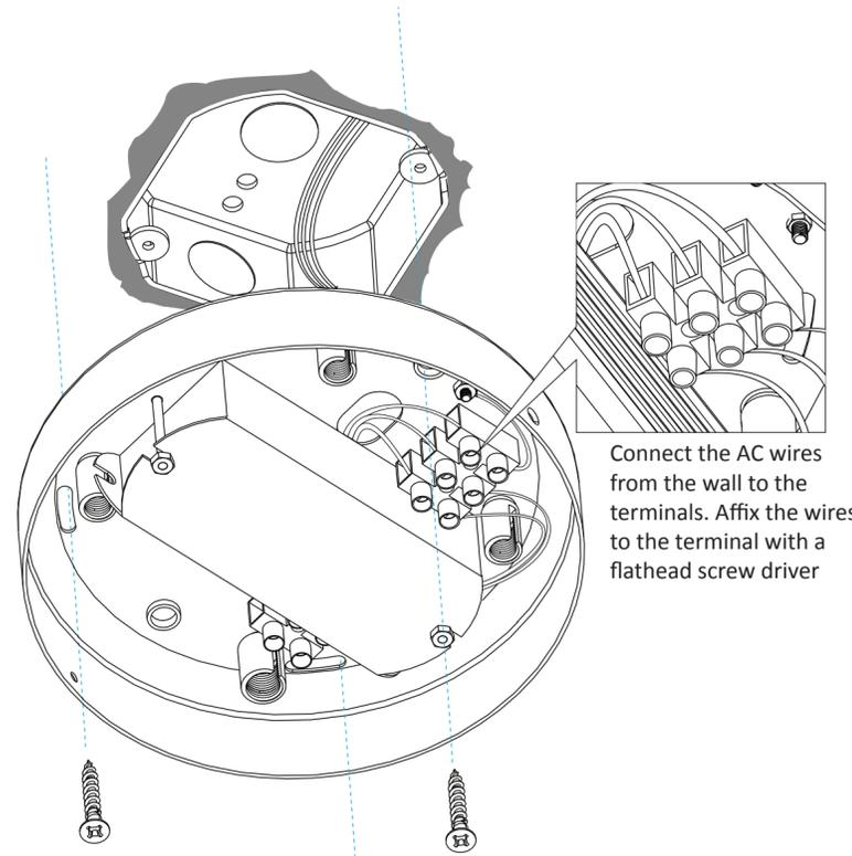
Connect the AC wires from the wall to the terminals. Affix the wires to the terminal with a flathead screw driver
