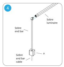
Make sure the plug of the Sobre end bar is facing inward and in the same direction as the wider side of the mounting block. Plug in luminaire to the end bar (refer to Sobre user manual for further lamp assembly instructions).
