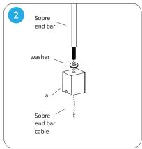
Insert the Sobre end bar into the hollow tube of the mounting block. If the end bar comes with a cable, feed the cable through the tube before inserting.
