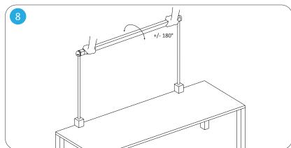
The luminaire can be turned 180 degrees each way to aim the light in the desired direction.
