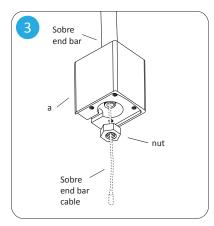
Secure the Sobre end bar to the mounting block with the nut retained from Step 1 using a pair of needle-nose pliers.
