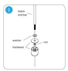
Remove the hardware from the Sobre end bar(s). Leave one washer for use in step 2.
