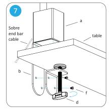
Sit the mount on the edge of the table. Attach the screw handle to the clamp piece with the short screws.
