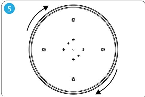
Once the Ramen wall sconce is inserted onto the backplate on the wall, rotate it clockwise until it clicks into place.
