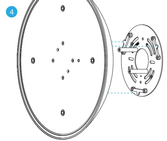
Insert the Ramen wall sconce onto the backplate on the wall by aligning the slots. Align the slots where the red dots are.
