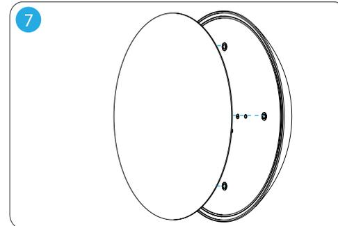
Finally, magnetically put on cover plate. (note: you may remove cover plate by using the provided magnet.)
