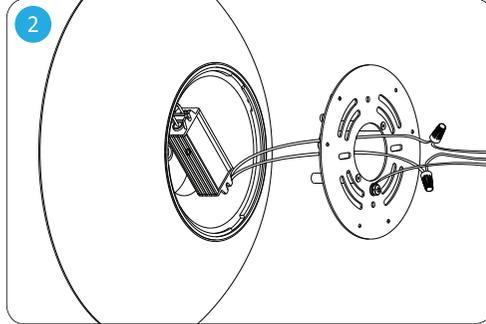
Using the provided cable connectors, connect the wires. Attach ground wire to the green screw on the unit.
