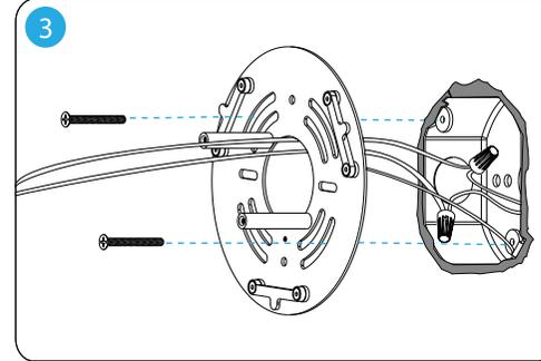
Secure the back plate of the Ramen wall sconce to the junction box with the provided screws.
