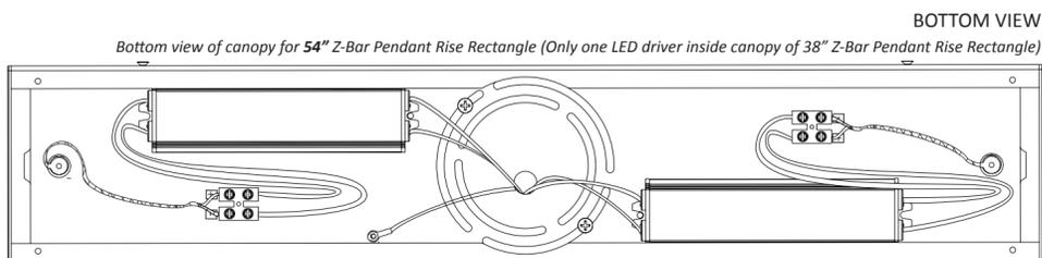
Bottom view of canopy for 54" Z-Bar Pendant Rise Rectangle (Only one LED driver inside canopy of 38" Z-Bar Pendant Rise Rectangle)
