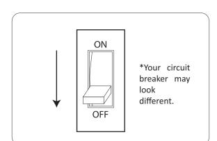
Shock Hazard. Electric shock could result in serious injury or death. Make sure circuit breaker is set to OFF before installation. Must be installed by a qualified electrician.
