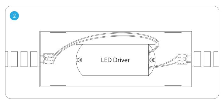
Using the provided DC cable & connectors, connect the wires inside the transformer enclosure as illustrated in the Wiring Diagram below.
