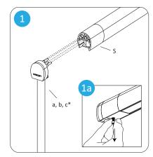
Push the end bars into the luminaire. If you experience difficulty pushing the bars into the luminaire, make sure the hex screw is disengaged. To disengage the hex screw, loosen up the screw using the provided hex key, and then pull down the screw (see 1a)
