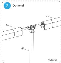
Push the connecting bar(s) into the luminaires to connect the modules. If you experience difficulty pushing the bars into the luminaire, make sure the hex screw is disengaged. To disengage the hex screw, loosen up the screw using the provided hex key, and then pull down the screw (see 1a)
