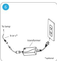
Connect the transformer to the lamp cable, then plug in the transformer to the wall outlet.
