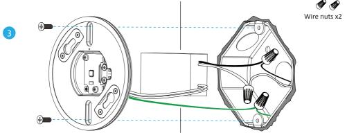
Using the provided wire nuts, connect the Live (black) wire to the Live wire from the mains, the Neutral (white) wire to the Neutral wire from the mains, and the Ground (green) wire to the Ground wire from the mains. Enclose the LED driver inside the wiring box. The wiring (junction) box must be large enough to accommodate the LED driver (2 ¾" x 1 5/8" x 7/8"). The following wiring boxes have been tested and confirmed to be compatible with this installation:
