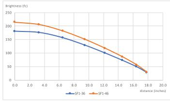
Photometrics: light source placed 19" away from work surface
