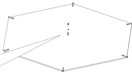
Locate the center location of the hexagon panel. Using the provided short screw and a screw driver, affix the holder to the center location. Then, fit the provided wire through the cable gripper and screw the cable gripper into the holder.
