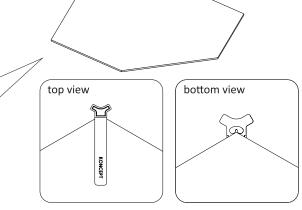
Secure the clear plastic holder with screws to a corner of the hexagon acoustic panel. Make sure the protruding part of the clear plastic holder is sitting tight against the corner of the panel (see bottom view). Repeat the same for all 6 corners. Be sure not to overscrew as it may damage the acoustic panel and the screws would not be able to be securely mounted.
