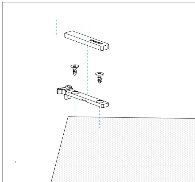
Secure the clear plastic holder with screws to a corner of the square acoustic panel. Make sure the protruding part of the clear plastic holder is sitting tight against the corner/edge of the rectangle acoustic panel. Repeat the same for all 4 holders. Be sure not to overscrew as it might damage the acoustic panel and the screws would not be able to be securely mounted.
