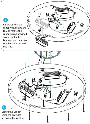
Connect all 3 sets of Hot, Neutral and Ground per illustrated and affix LED drivers to the junction box. Further support the canopy by evenly screwing on supporting screws.
