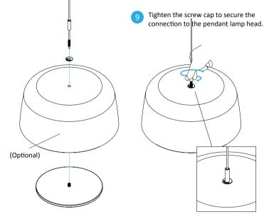
Connect the cable to the pendant head.
