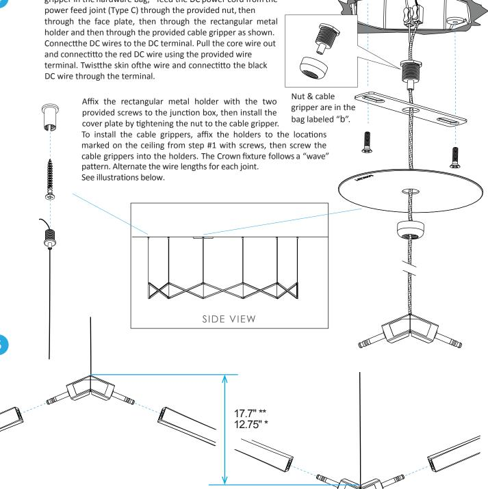
Attach the LED light bars to the joints making sure they are fully inserted with no gaps between the light bars and the joints. Ensure every joint is positioned so that its center opening is always facing inward, and not upward, downward or outward of the entire fixture.
