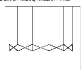
the ceiling according to the measurements shown below. The Z-BAR pendant light will be hung vertically from each of the joints.
