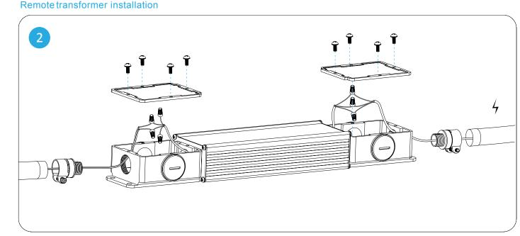
Using the provided DC cable & connectors, connectthe wires inside the transformer enclosure as illustrated in the Wiring Diagram
