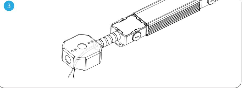
Feed the Red and Black DC wires through the conduit into the junction box (conduit and junction box not provided). Affix the transformer enclosure and junction box properly inside the ceiling, with an opening allowing access to the junction box.
