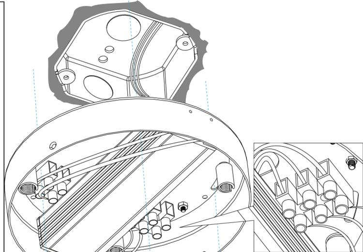
Connect the AC wires from the wall to the terminals. Affix the wires to the terminal with a flathead screw driver
