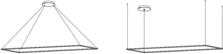
There are two ways to mount the Z-Bar pendant rectangle, a monopoint installation or a multipoint installation. For monopoint installation, proceed to step 2. For multipoint, see below.
