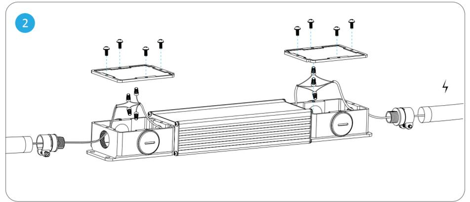
Using the provided DC cable & connectors, connect the wires inside the transformer enclosure as illustrated in the Wiring Diagram below. A transformer needs to be installed for every location marked with the symbol Ⓝ
