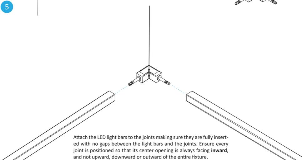
Attach the LED light bars to the joints making sure they are fully inserted with no gaps between the light bars and the joints. Ensure every joint is positioned so that its center opening is always facing inward, and not upward, downward or outward of the entire fixture.
