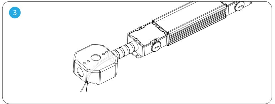
Feed the Red and Black DC wires through the conduit into the junction box (conduit and junction box not provided). Affix the transformer enclosure and junction box properly inside the ceiling, with an opening allowing access to the junction box.
