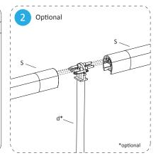
Push the connecting bar(s) into the luminaires to connect the modules. If you experience difficulty pushing the bars into the luminaire, make sure the hex screw is disengaged by loosening up the screw using the provided hex key and pulling down the screw.
