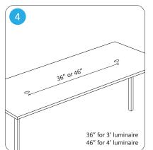
Drill two or more 7/16" diameter holes as needed in the table. Center the hole placement on the table, making sure the holes for the 3' luminaire are 36" apart, and holes for the 4' luminaire are 46" apart.
