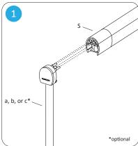
Push the end bars into the luminaire. If you experience difficulty pushing the bars into the luminaire, make sure the hex screw is disengaged by loosening up the screw using the provided hex key and pulling down the screw.
